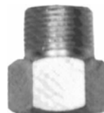
10732 - CONE ADAPTER For adopting vent cop fittings. 1" . 14 UNS(m) X 7/8" . 14 UNF(f) cone.
